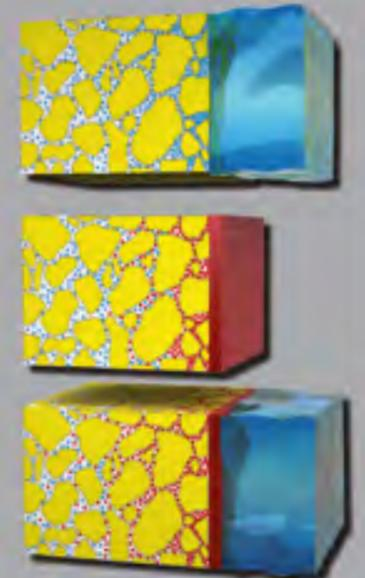
**CRYSTALLIZATION AND SEALING OF CAPILLARY NETWORK FOR CONCRETE**
