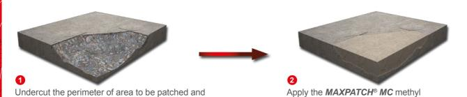
methacrylate patching mortar.
