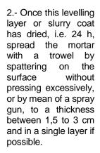
If greater thickness is required, allow one day before applying another layer over it, which will previously be left rough to ease the bonding of the next one. For finishing procedures it can be smoothed with an aluminium straight edge or metal trowel, without pressing excessively so as not to reduce the porosity of the mortar.
