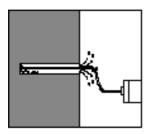
For removing the dust, clean the hole by brushes and blowing-out devices. Make sure that threaded rods or rebars are free of any contaminants, oils, greases, dust, etc.
