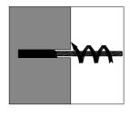
In order to get a good impregnation of the anchors, threaded rods or rebars with epoxybased resin into the hole, a light twisting motion should be done while those are placed. Make
